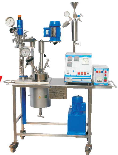
2L instrument with separate head for weight loss method & electrochemical corrosion studies
